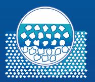
Seal-O-Crete penetrates into the concrete where it reacts with free lime and alkali to fill the voids and bond the particles into a solid mass, creating a permanent seal.
